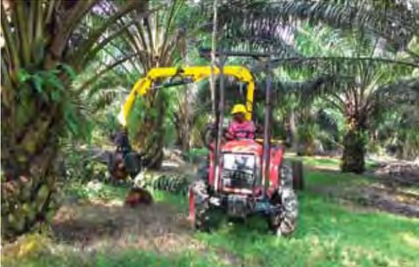
MTG is used to load FFB
