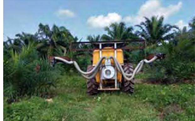
Power Sprayer is used to replace manual pesticide spraying
