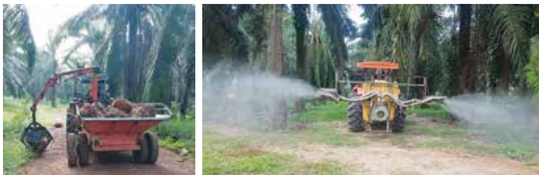
Photo 29 - (Left) Machinery used to collect FFB in the field, (Right) Blast sprayer helps to maximise chemical coverage
